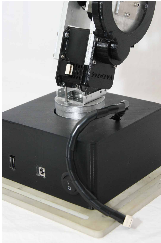
Figure 2.3: Correct placement of the arm into the baseplate motor bracket.
