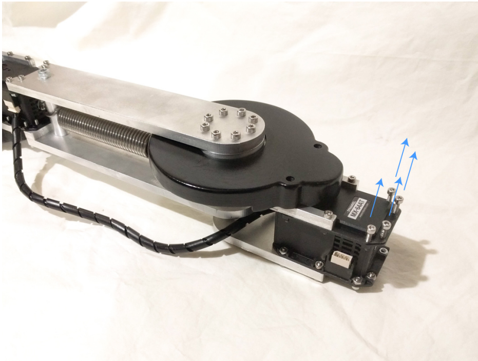
Figure 2.2: Remove screws attached to base
