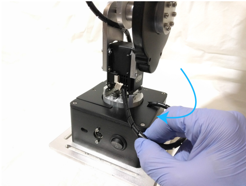
Figure 2.4: Install the cable from the baseplate into the lower arm motor.
