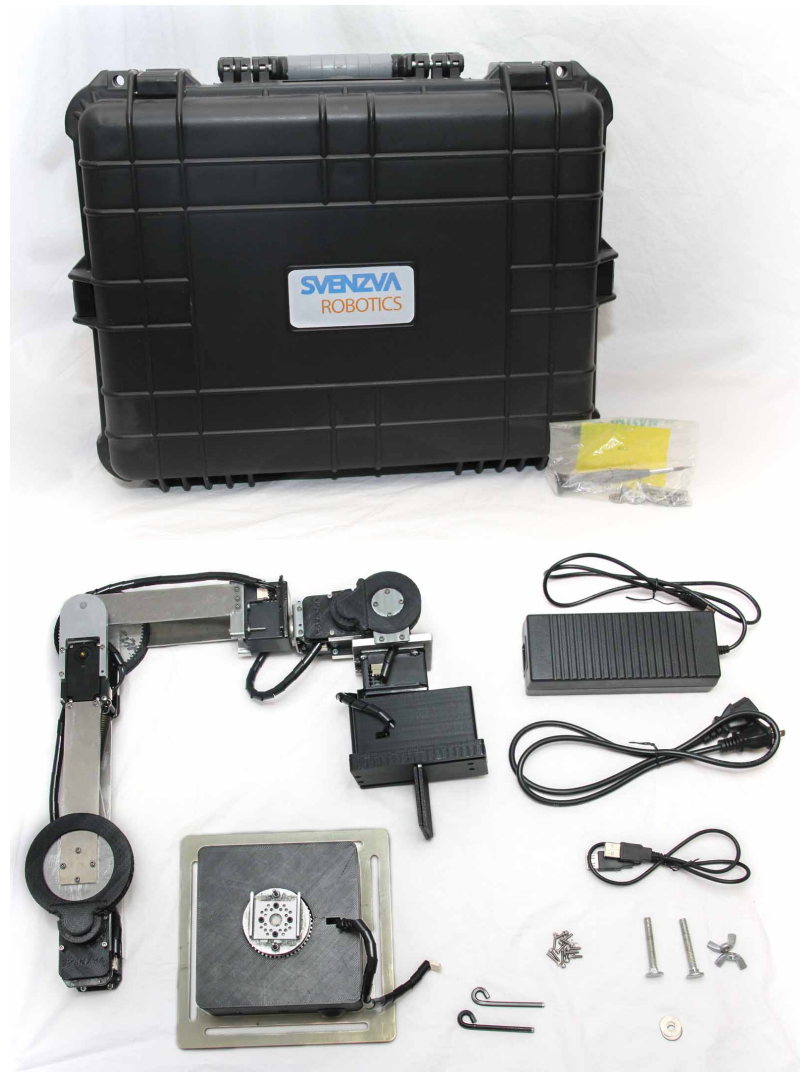
Figure 2.1: Included contents of a shipped Revel platform: carrying case containing the robot & cables, and an assorted hardware pack
